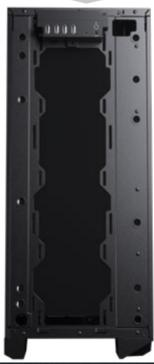
The left-side fan bracket can be installed in a secondary position to pull air from the front of the chassis. Secure the fan bracket with 5x screws as shown.
